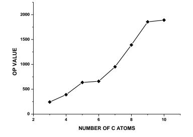
Figure 6: Plot of the number of carbon atoms vs. OP value for cycloalkanes with a single ring.
